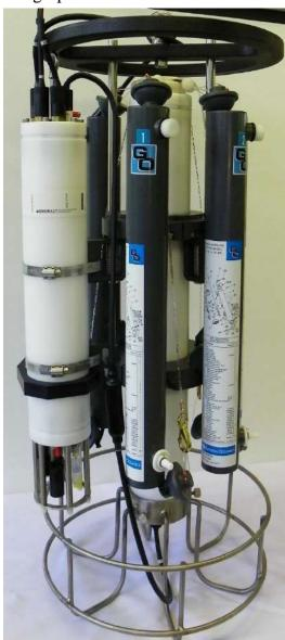
integrates a rechargeable battery pack to power the sampling system and the interfaced CTD. Instead of a bottle it is possible to install an IDRONAUT OCEAN SEVEN CTD, (OS310, OS316Plus or OS320Plus) which takes control of the MISS sampling system operations and provides real-time measurements from the installed sensors like but not limited to: Pressure, Temperature, Conductivity, Salinity, pH, Dissolved Oxygen, Redox, Turbidity, Chlorophyll-a, Phycocyanin, Phycoerythrin.
